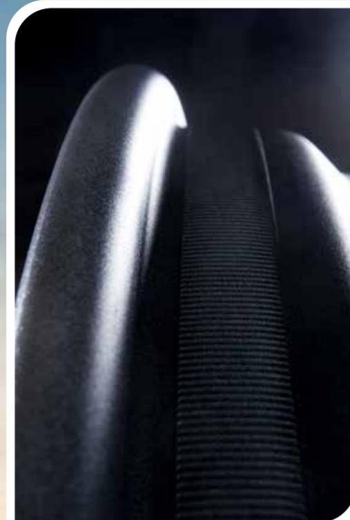
The knurling has been increased by 50% compared to the standard version. This, combined with the special friction paint, maximises the friction characteristics of rim when the tire is fitted.
