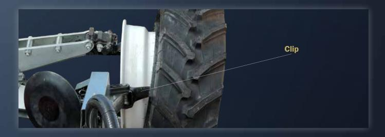
• Move the clip of the tire fitting machine in the front part of the rim to perform the fitting of the second bead.
