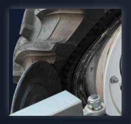
• Lubricate the Red Rubber Spacer with a brush, using the proper mounting paste.
