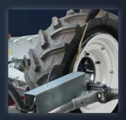
• Rotate the PneuTrac® until the disc plate remove on the front side is approximately 180° from the midpoint between the two clamps on the rear side.
