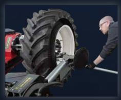
When the second bead is completely detached from the rim, remove the clip from the bead • Continue to **turn the spindle very slowly** counterclockwise while raising up the clip.
