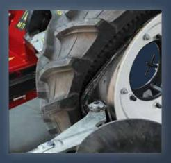
• Rotate the PneuTrac® slowly until the clip on the front side is at 0° position relative to the midpoint between the two clamps on the back side.
