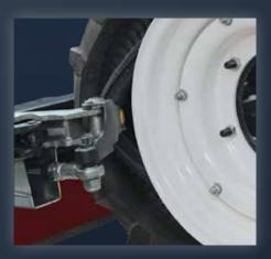
• During this operation, move the clip back and forth in the gap between the rim and the bead every few centimeters.
