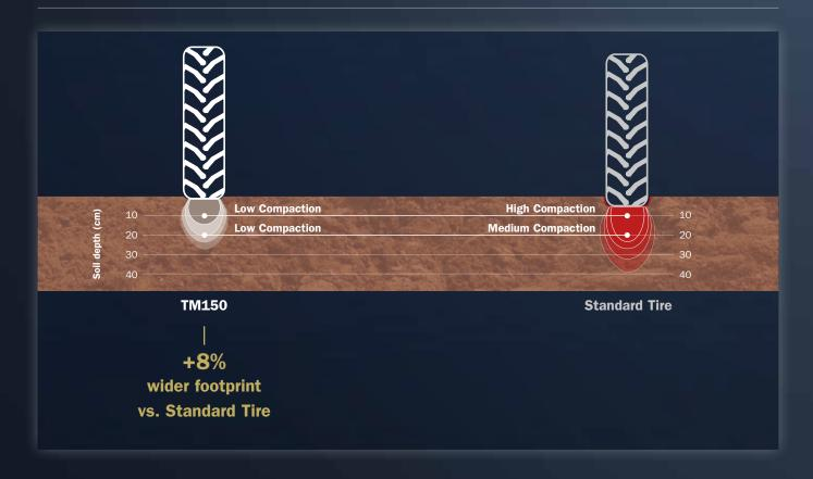
As you go deeper into the soil, the standard tire causes compaction that worsens rapidly. At 20cm depth, the TM150 maintains "low" compaction, while the standard tire is already experiencing "medium" compaction.
